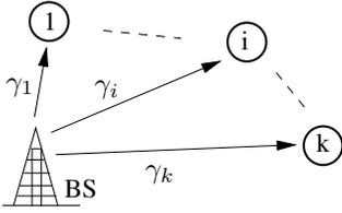
Fig. 1. A system consisting of a BS and  $k$  mobile users. Each user  $i$  sets its timer depending on its SNR  $\gamma_i$ .
