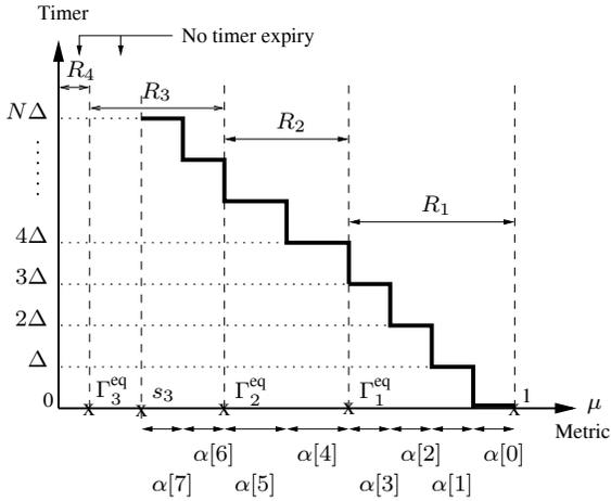
Fig. 3. Illustration of the optimal timer mapping for  $N = 8$  slots and  $M = 4$  rates. It shows that  $r_1 = 4$  equal length intervals occupy the entire interval  $[\Gamma_1^{\text{eq}}, 1)$  for which the rate is  $R_1$ . Similarly,  $r_2 = 2$  and  $r_3 = 2$ . Furthermore,  $\Gamma_3^{\text{eq}} \leq s_3 < \Gamma_2^{\text{eq}}$ .
