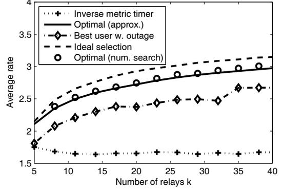
Fig. 4. Average rate (in bits/symbol) as a function of  $k$  when  $N = \lfloor \frac{T_{\text{max}}}{\Delta} \rfloor = 10$  ( $R_1 = 4$ ,  $R_2 = 3$ ,  $R_2 = 2$ , and  $R_1 = 0$ )
