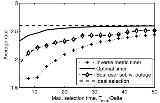
Fig. 5. Average rate (in bits/symbol) as a function of  $T_{\text{max}}/\Delta$  when  $k = 10$  ( $R_1 = 4$ ,  $R_2 = 3$ ,  $R_2 = 2$ , and  $R_1 = 0$ )
